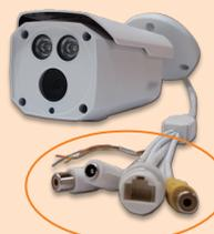
IP cameras with pigtail may generate more interference and intensify the degradation of electrical signals.
