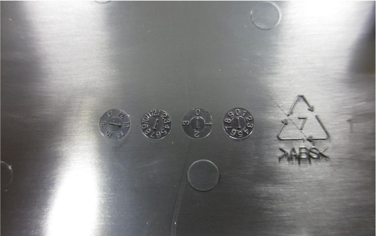
The main material of enclosure is ABS material.
