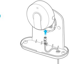
(5) Attach the AP to the inner case by rotating ti in a clockwise direction until it clicks into place.
