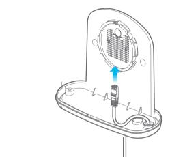
(5) SAlign the mounting holes on the bracket with the inner case. Secure the bracket to the inner case with two screws. Slide the AP down the bracket until it clicks into place.
