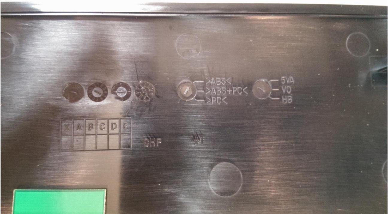
The main material of enclosure is ABS material.
