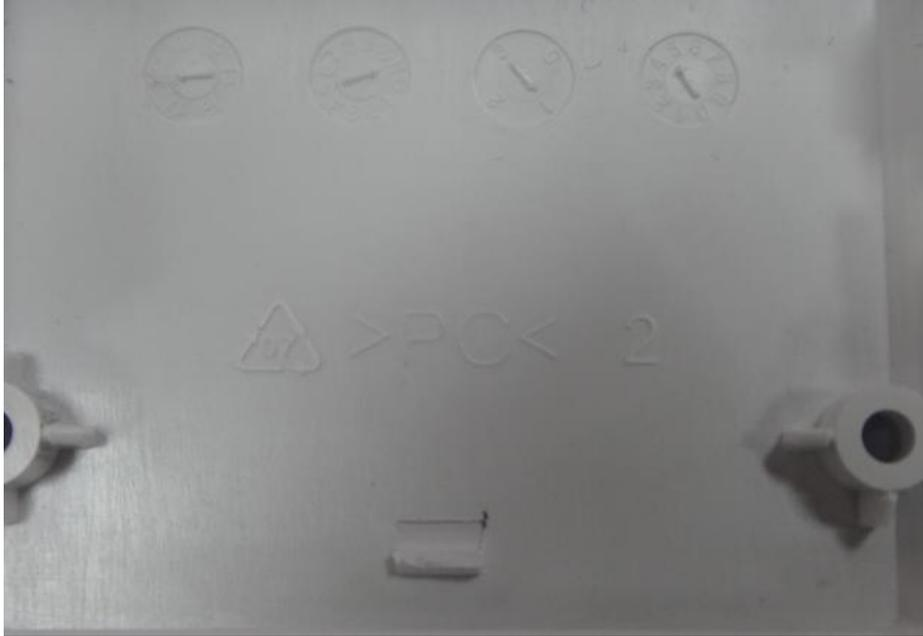
The main material of enclosure is PC material.
